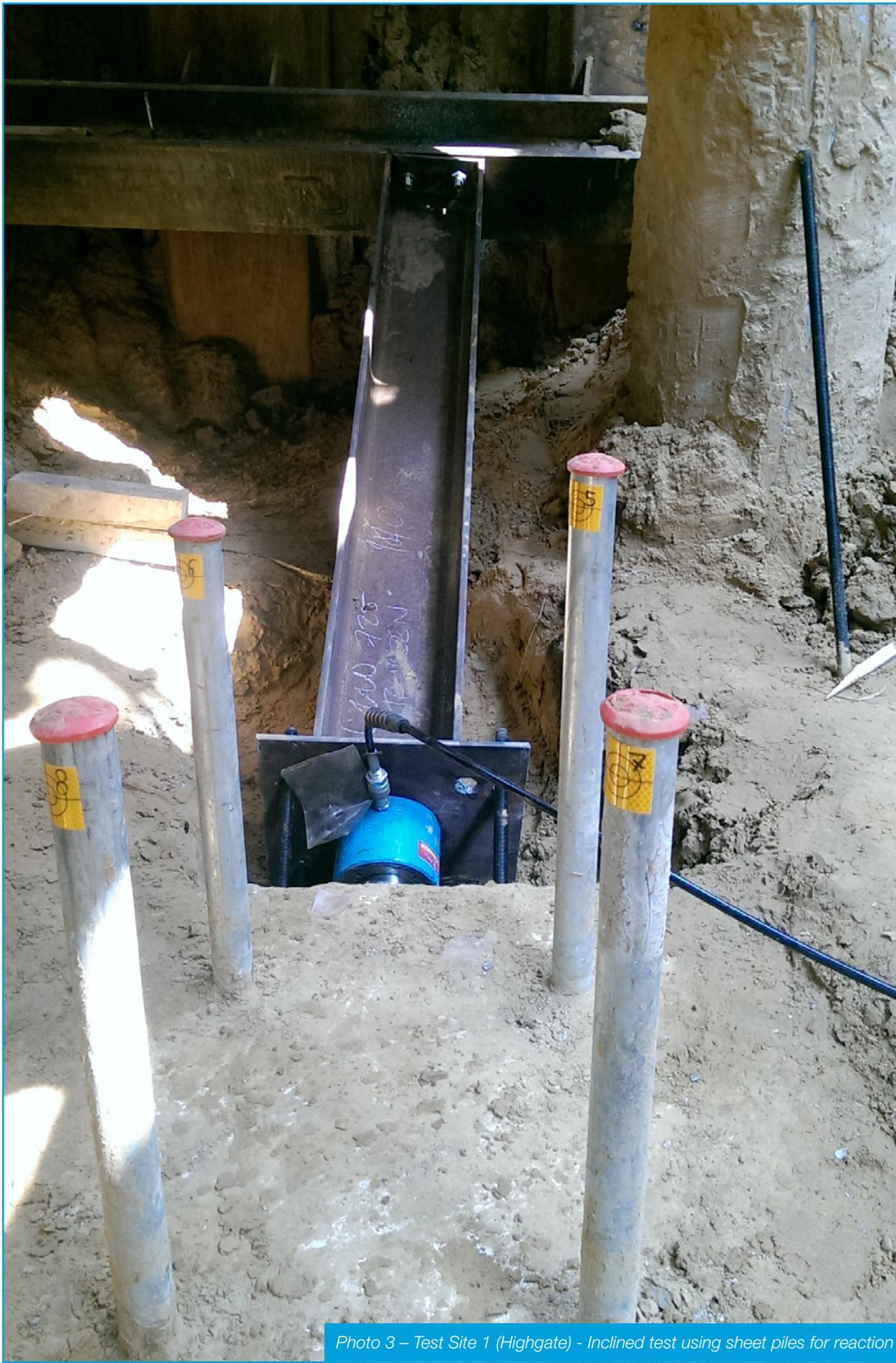
Photo 3 – Test Site 1 (Highgate) - Inclined test using sheet piles for reaction
