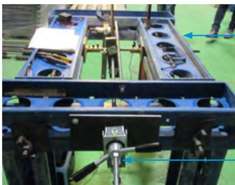
Frame and stand made from proprietary soldiers (e.g. RMD or similar), which can be bolted together with proprietary corner brackets or tied together with ties.
