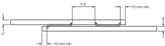
Figure 5 — Start and finish of a lap joint
