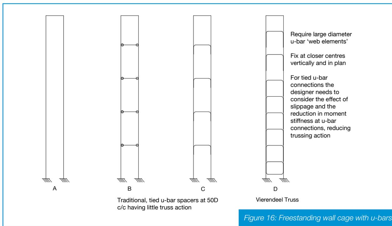
Figure 16: Freestanding wall cage with u-bars
