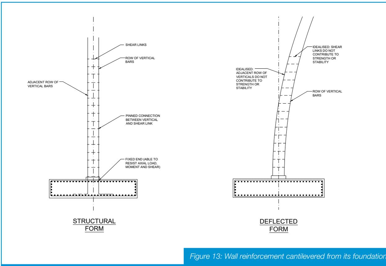
Figure 13: Wall reinforcement cantilevered from its foundation
