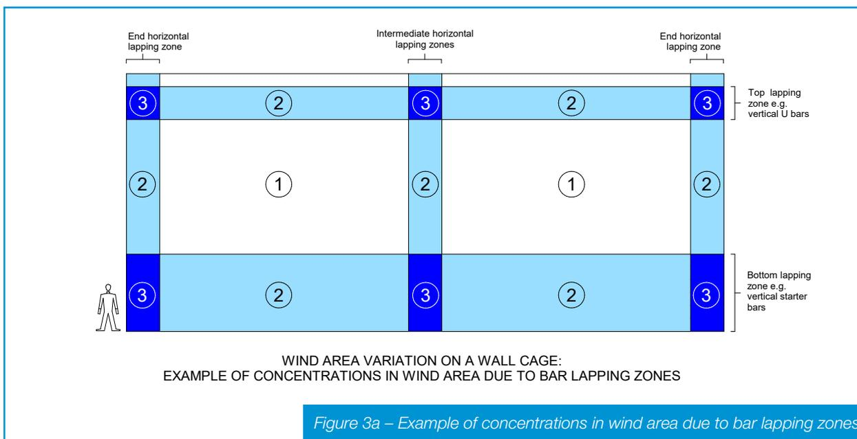
Figure 3a – Example of concentrations in wind area due to bar lapping zones
