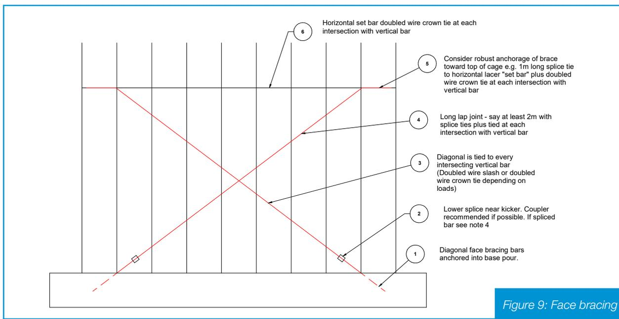
Figure 9: Face bracing
