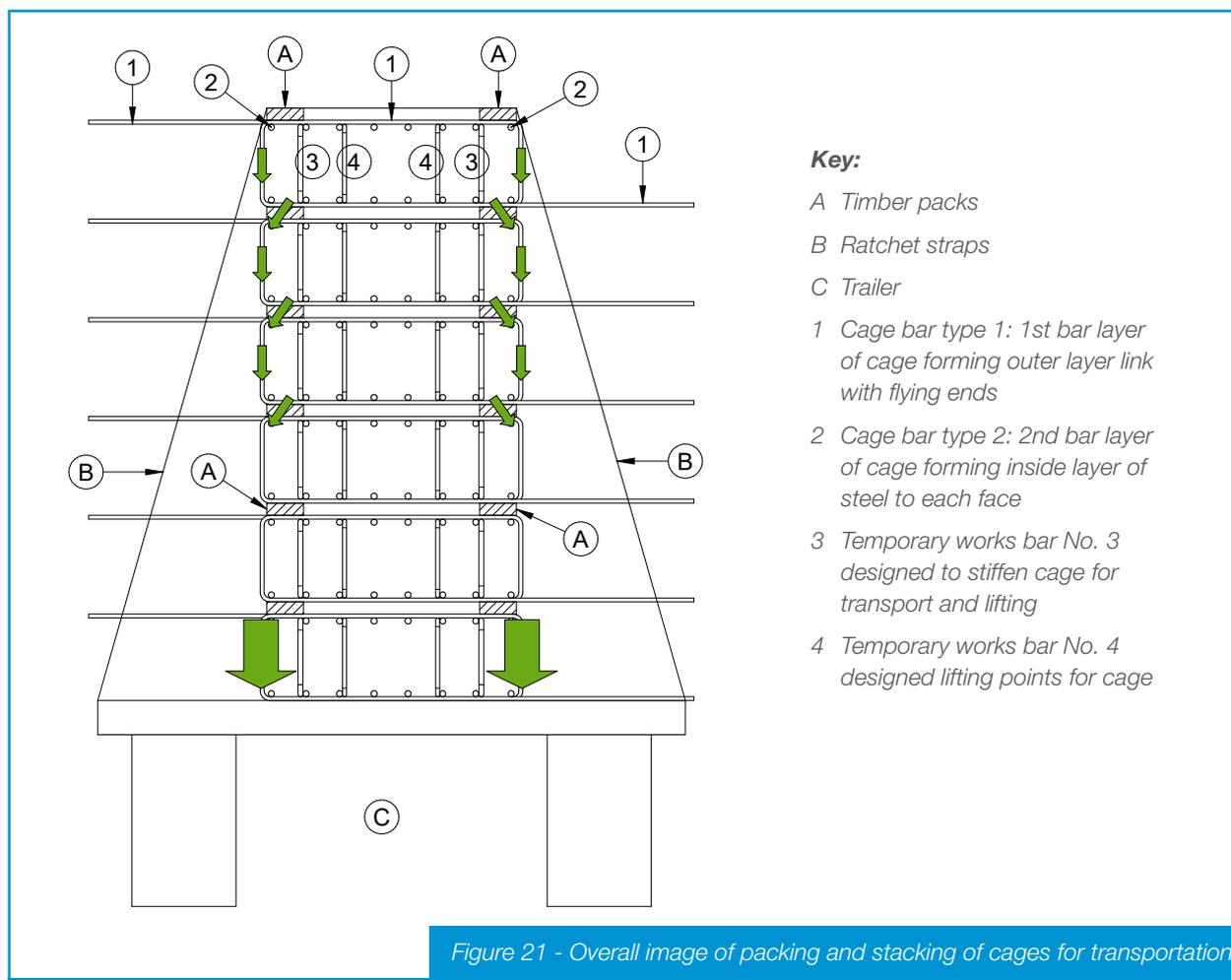
NOTES: Temporary works design requires packs as indicated. These packs span across the top of all the outer links (bar No.1). The packs must be as close to the vertical legs of links (bar No.1) as possible.
