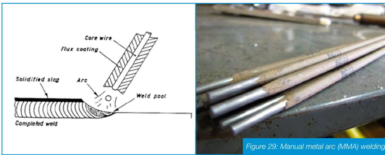
Figure 29: Manual metal arc (MMA) welding
