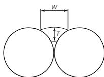
For ease of inspection on site, a conservative estimate of the effective throat thickness may be taken as  $\frac{W}{2}$ .
