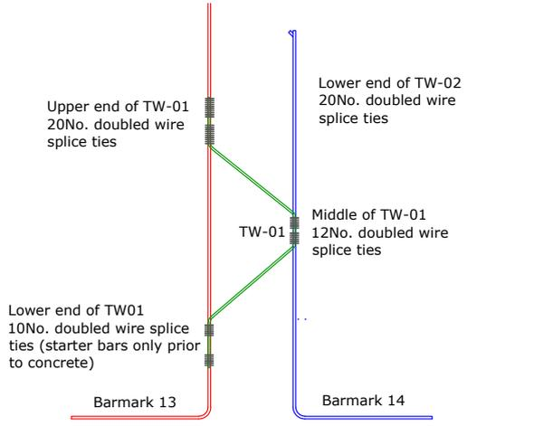
NOTE: To provide 'truss action' Barmark TW-01 (SC46) must be rigidly connected to both Barmarks 13 and 14. This is shown achieved using doubled wire, wrapped splice ties distributed along the parallel splice legs.
