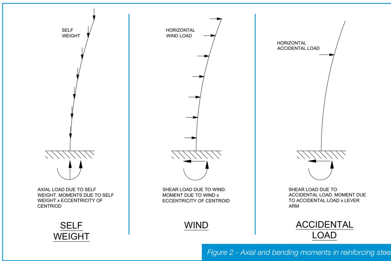
Figure 2 - Axial and bending moments in reinforcing steel
