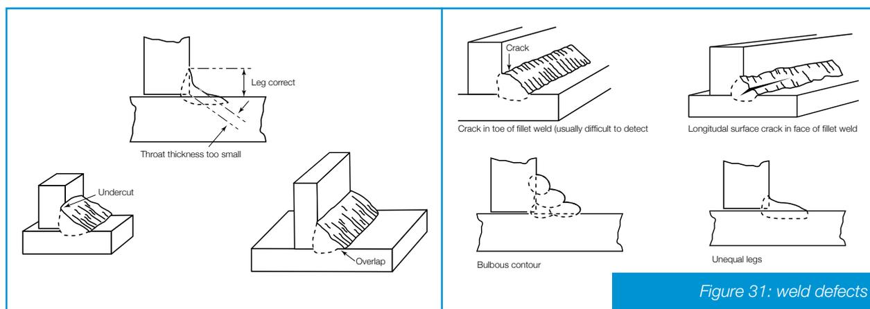
Figure 31: weld defects
