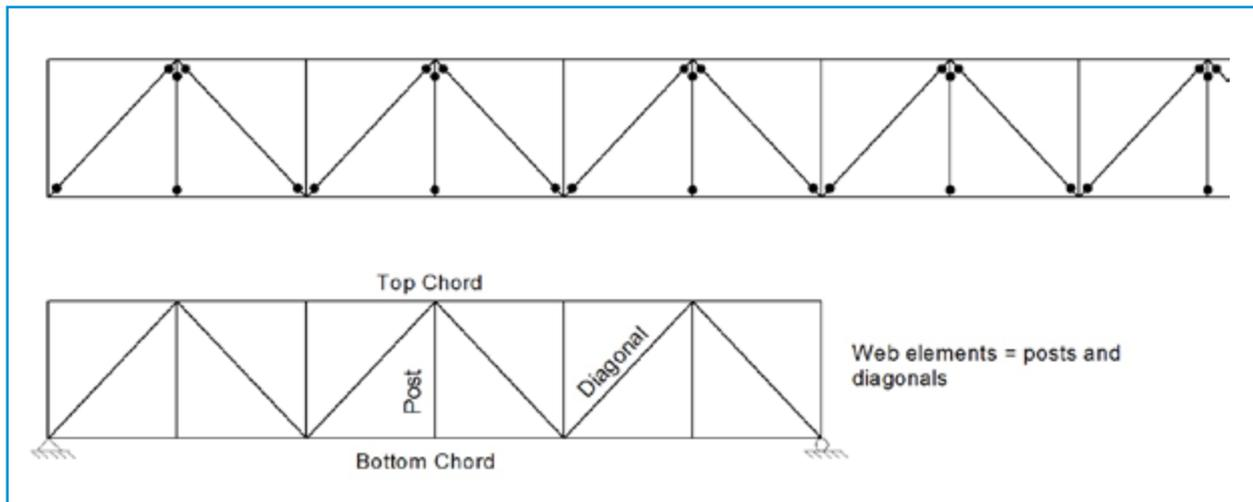
Figure 10: Truss terminology with cage orientated as a beam
