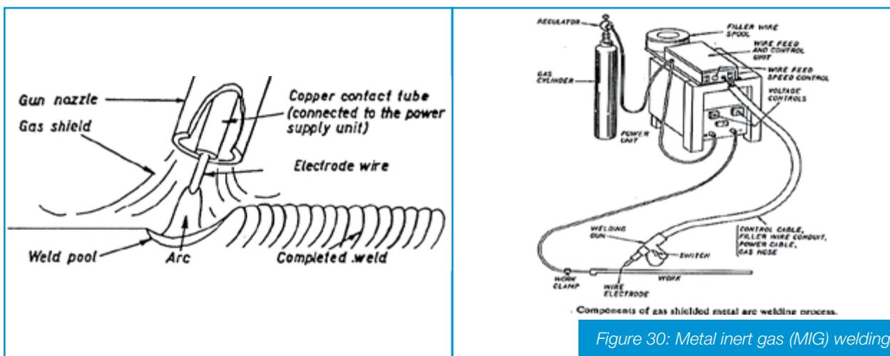
Figure 30: Metal inert gas (MIG) welding
