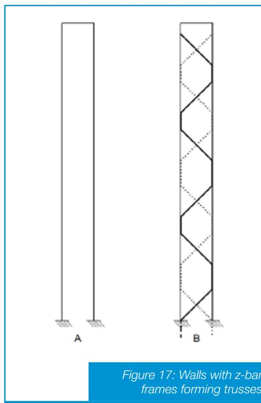
Figure 17: Walls with z-bar frames forming trusses
