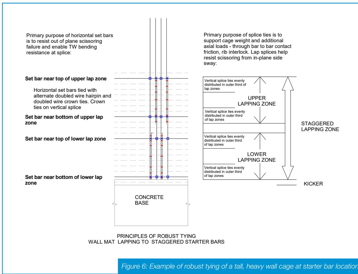
NOTE: If ties are used to carry a higher proportion of their failure load, they stretch and become loose if load reversal occurs. This is discussed further in Method B.
