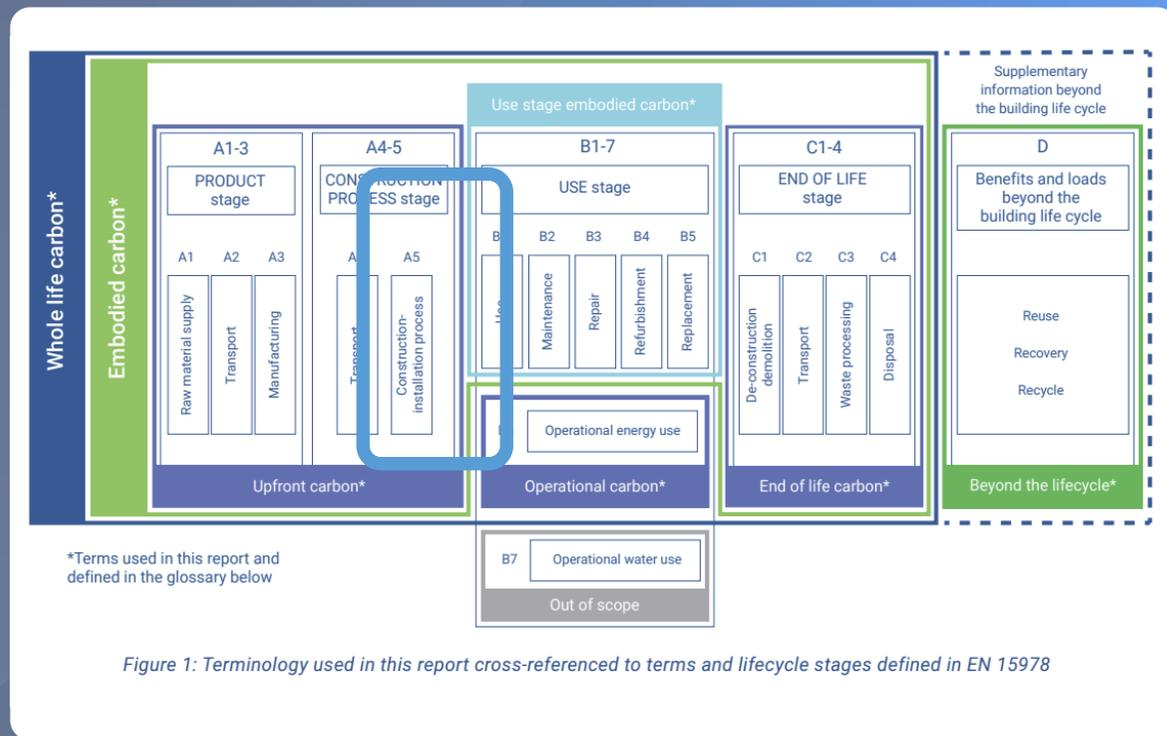
Figure 1: Terminology used in this report cross-referenced to terms and lifecycle stages defined in EN 15978
